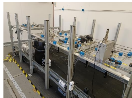
Figure 17: ESPRIT and VV BBM Fluidic Panels with Mass Flow Meter (right)
