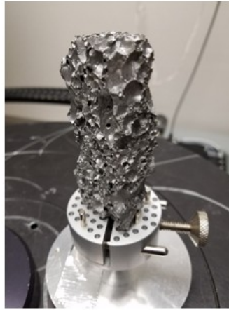
Figure 10. Early prototype version of cold CT setup at NASA GSFC (newer version uses more insulative materials). Cold immersive environmental chamber is allowed to rotate underneath fixed cryogenic feed lines. Sample shown here was a block of aluminum foam, cooled under N_2 at -100 degrees C.
