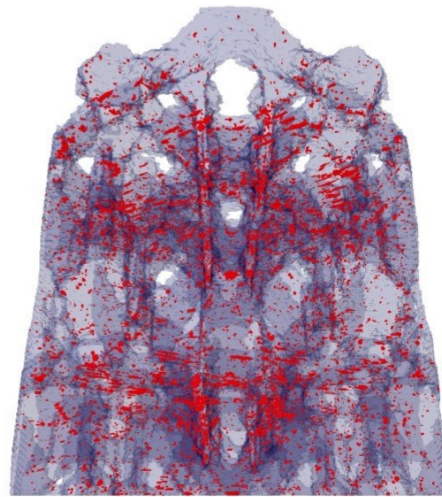
Figure 15. Internal porosity segmented from external air surrounding an aluminum truss structure
