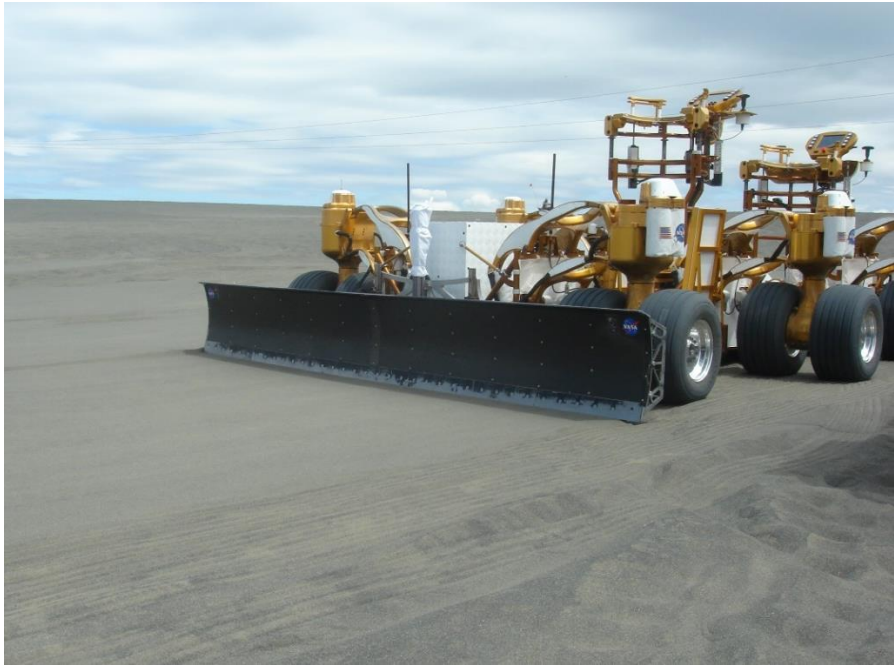
Figure 3. NASA Chariot rover with a bulldozer blade attached to it during Desert RATS field tests on sand dunes in Moses Lake, Washington.
