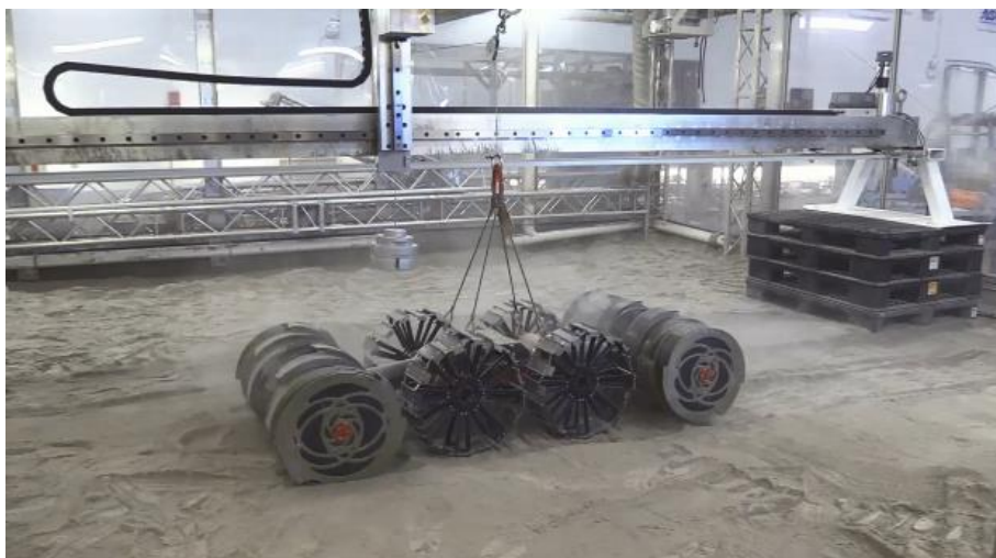
Figure 4. NASA Regolith Advanced Surface Systems Operations Robot (RASSOR) excavator undergoing gravity off-loading tests
