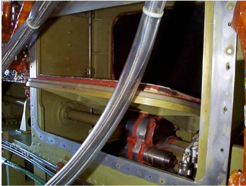
Figure 2: A Space Shuttle orbiters active vent, shown from the inside of the aft compartment.
