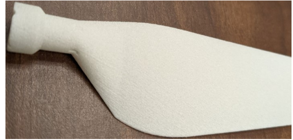
(b) SLS blades with noticeable surface roughness.
