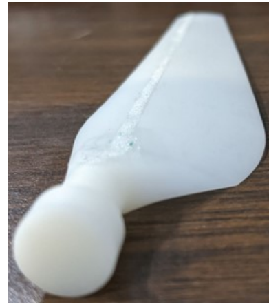
(a) SLA-tripped blades with adhered boundary layer trip.
