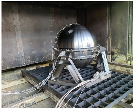
1 2 Figure 11: Top panel: A DAVINCI half-scale Engineering Test Unit (ETU) descent 3 sphere before a Venus environment test as part of the development of the overall 4 mission concept. Bottom panel: A full-scale DS ETU was tested to Venus 5 temperature profiles in Jan.-Feb. 2021, with successful verification of 6 performance at temperature. Diameter of the sphere is 0.98 m. Cables are 7 related to engineering testing apparatus. This ETU validated the descent 8 timeline temperature profile performance from ~70 km down to the Venus surface 9 during the DAVINCI mission Phase A activities.
