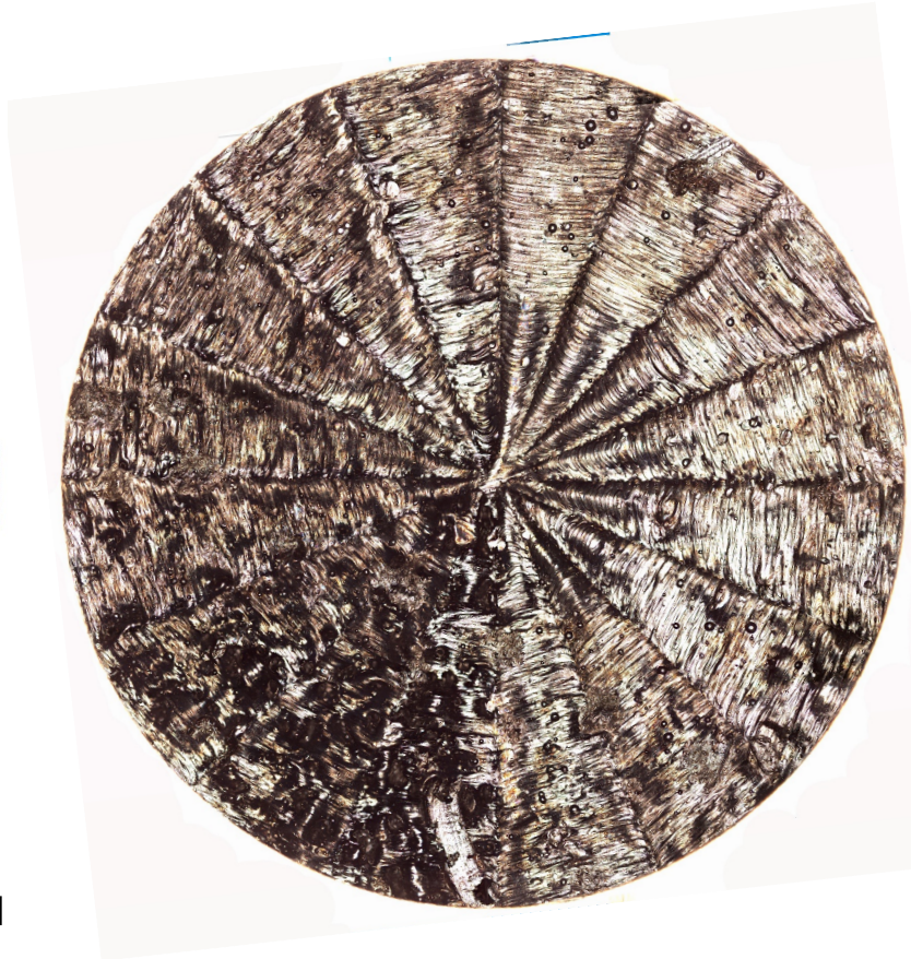
Microscope Image of the as printed surface
