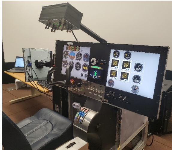
Fig. 7 The X-57 fixed-base piloted simulator.
