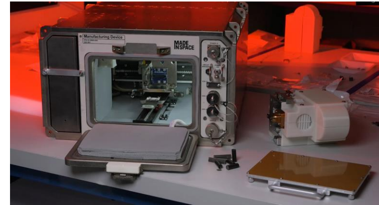
The Redwire Regolith Print facility suite, consisting of Redwire's Additive Manufacturing Facility, and the print heads, plates and lunar regolith simulant feedstock that will be launching to the International Space Station. Image Credit: Redwire Space, Inc
