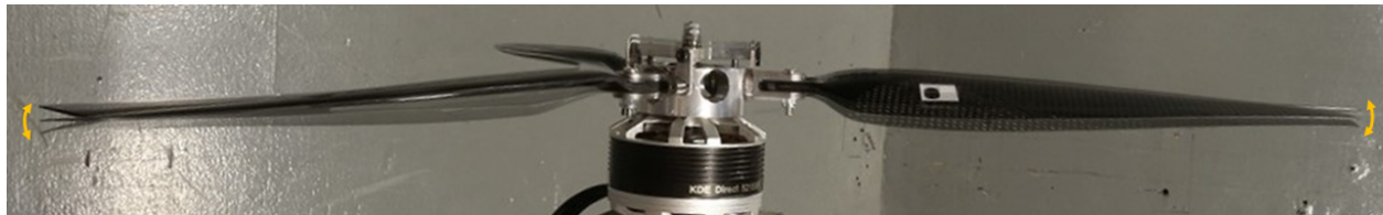
Fig. 4 Multi-exposure image showing propeller blade pitch movement.
