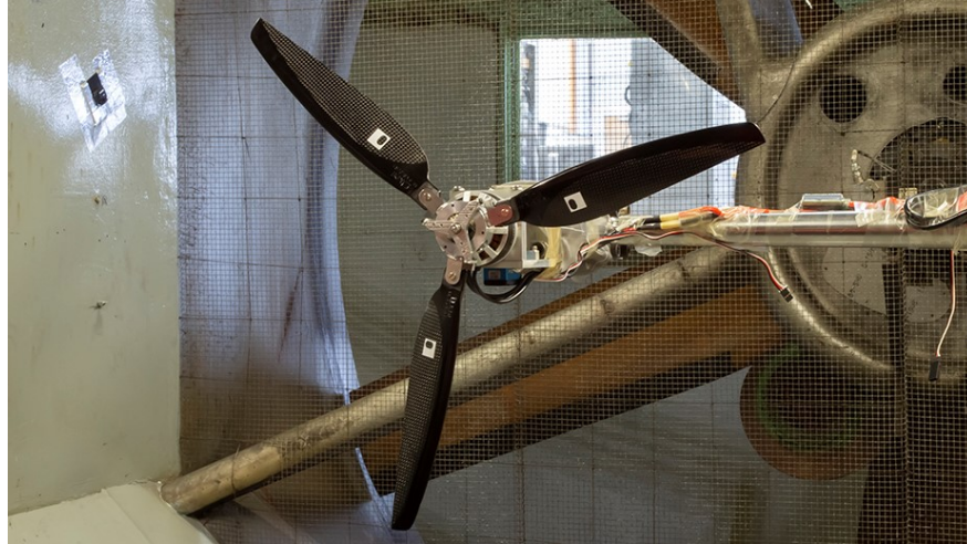
Fig. 3 Experimental propeller mounted on the wind tunnel sting.
