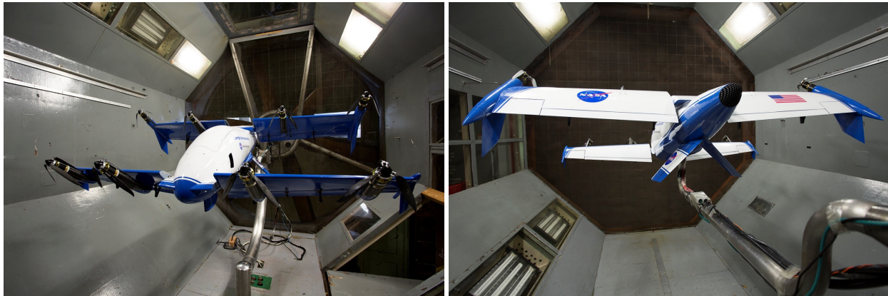
Fig. 1 LA-8 mounted in the NASA Langley 12-Foot Low-Speed Tunnel.
