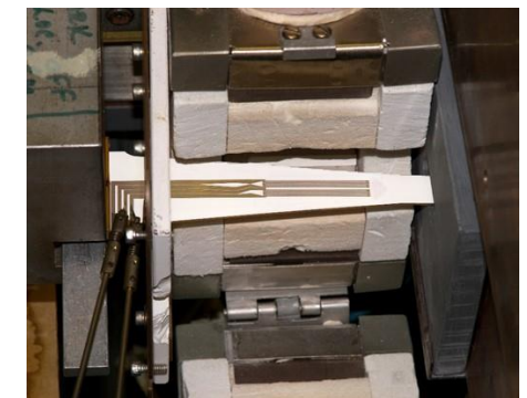
Specimen in fixture for Gf, TCR tests
