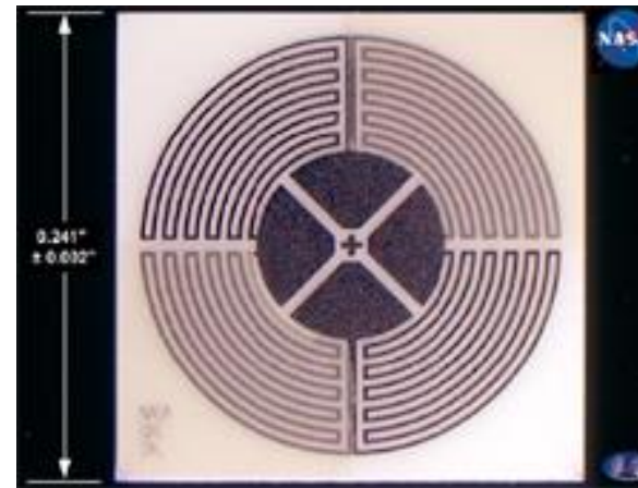
Heat Flux Sensor Array to T=1000^{\circ}\text{C}
