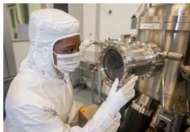
Ultra High Vacuum Metal Deposition System
