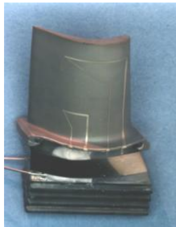
Pt- Pt/Rh temperature sensor to T=1200^{\circ}\text{C}
