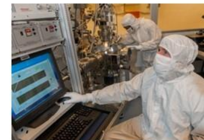
Tantalum Silicide Sputter Deposition System
