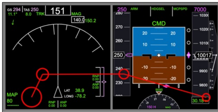
Figure 4: A close up view of a pilot’s eye shifting from the Primary Flight Display to the Navigational Display.
