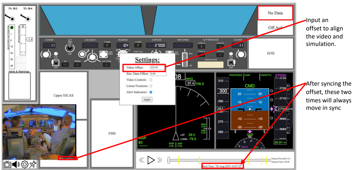
Figure 2: Input an offset to align the video and simulator data. In this case the offset is 422 seconds.
