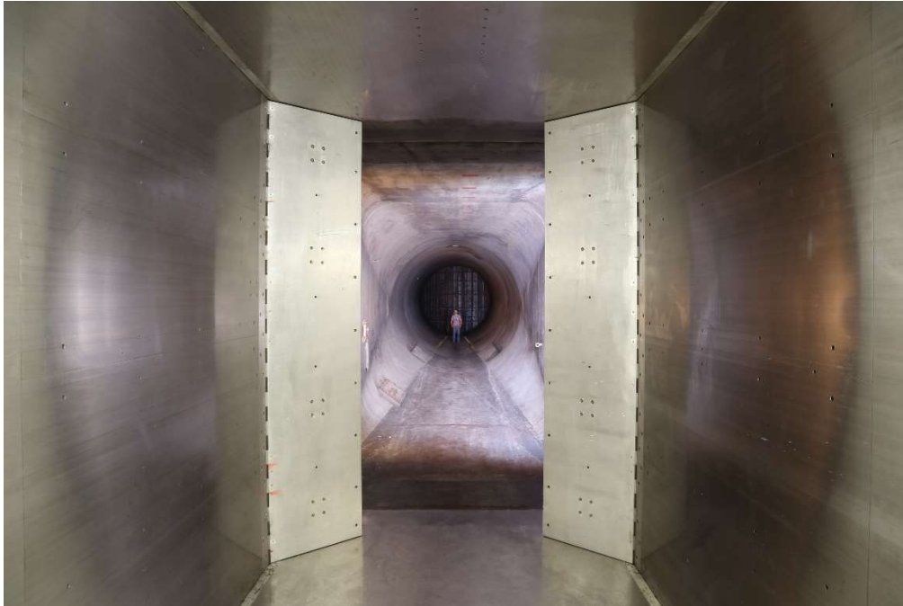
8x6 diffuser as seen from the test section looking downstream; visible person is halfway down
