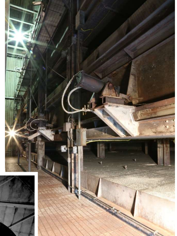
Air-dryer beds upstream of compressor with 8-layers of desiccant
