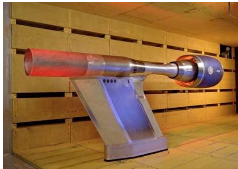
C-1994-01831L Turbfan model using compressed air as fan drive; installed in legacy 9x15 LSWT
