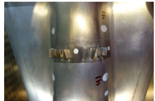
Three different vortex generator (VGs) installed for propulsion inlet testing
