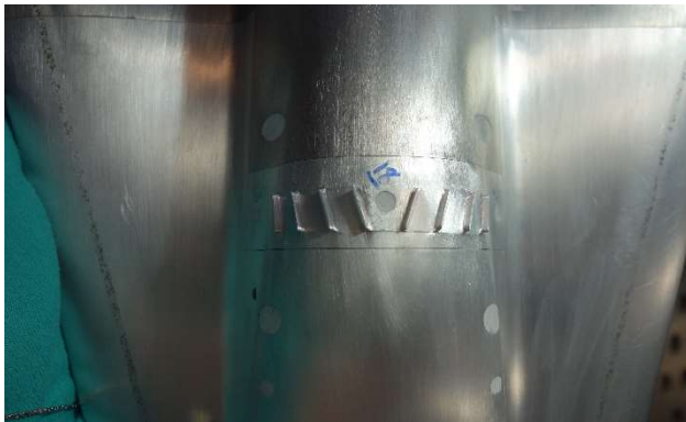
Three different vortex generator (VGs) installed for propulsion inlet testing
