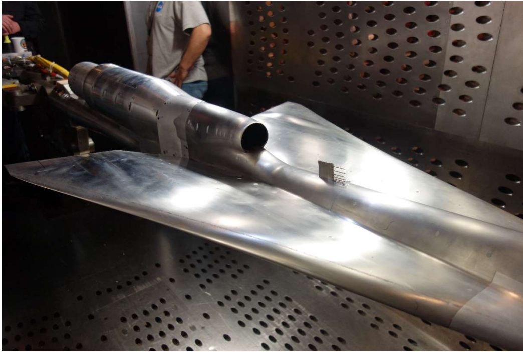
Three different vortex generator (VGs) installed for propulsion inlet testing
