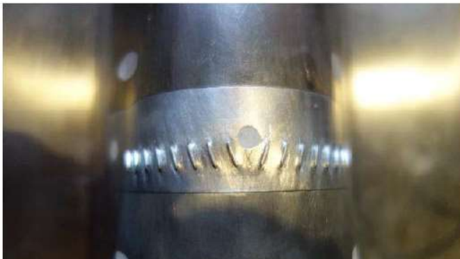
C607 Alternate, 16 VG's at 20° 0.053 in. high, 0.263 in. chord
