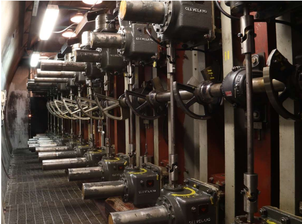
Hydraulic stations that drive a single wall and the cams that dictate wall movement
