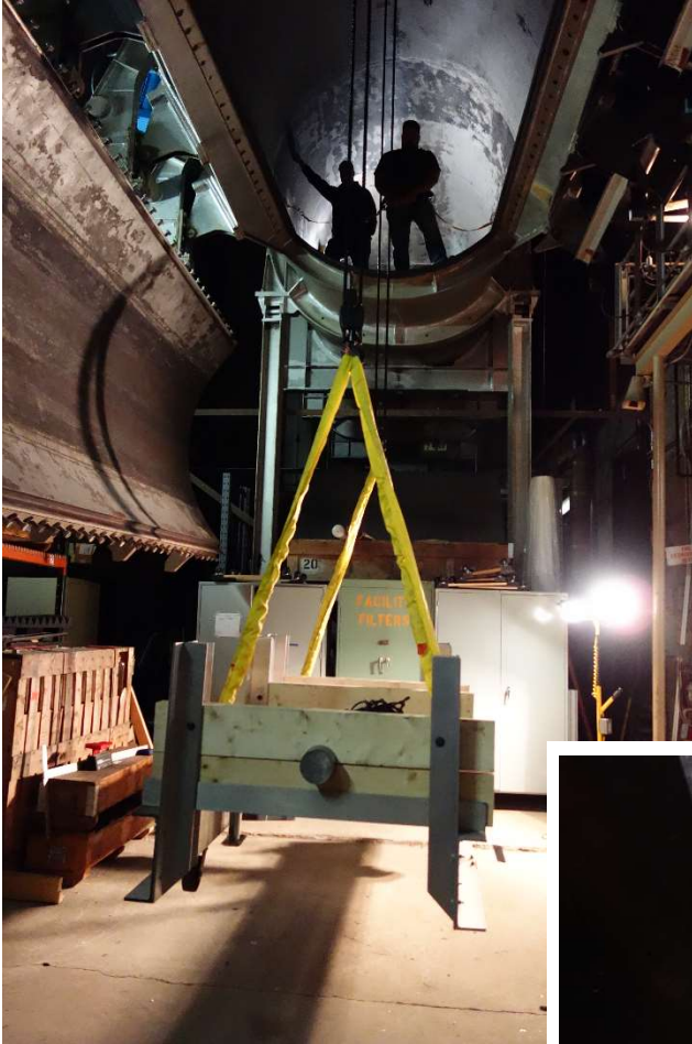
Lift of QueSST model into tunnel through downstream 16-foot hatch
