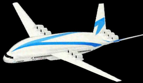
Center for High-Efficiency Electrical Technologies for Aircraft (CHEETA) Design Study for Hydrogen Fuel Cell Powered Electric Aircraft using Cryogenic Hydrogen Storage.
