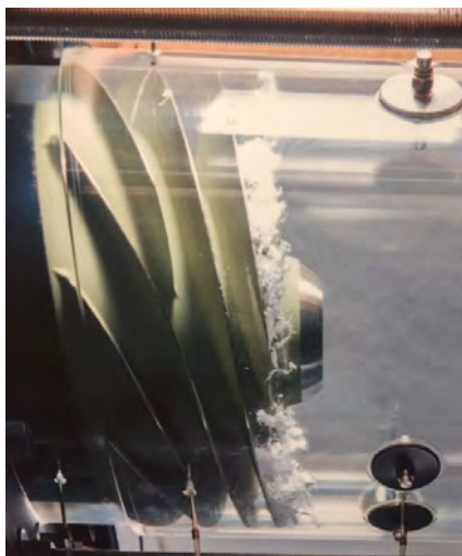
FIGURE 1. Inducer cavitation in water tunnel.
