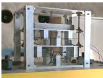
FIGURE 3. Experimental vibration isolation test bed attached to a shake table for dynamic testing. The rotational inertial device can be seen in the bottom middle of the test bed.
