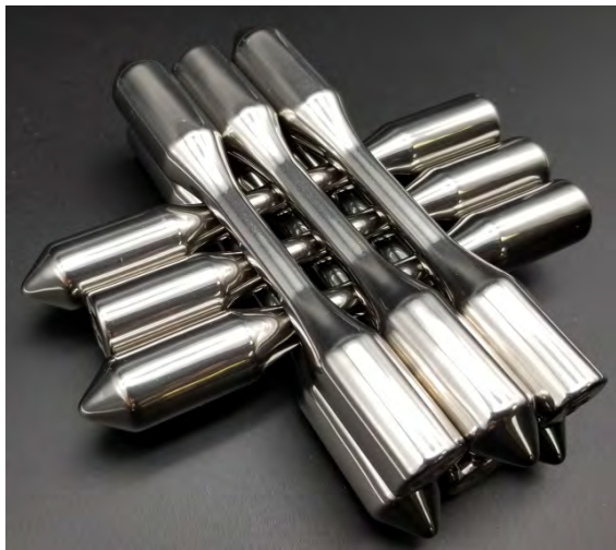
FIGURE 1. INCONEL 718 samples processed using CP/CMP surface enhancement from Phase I and II SBIR.
