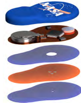
FIGURE 2. Cross-section of AstroSense printed sensor.
