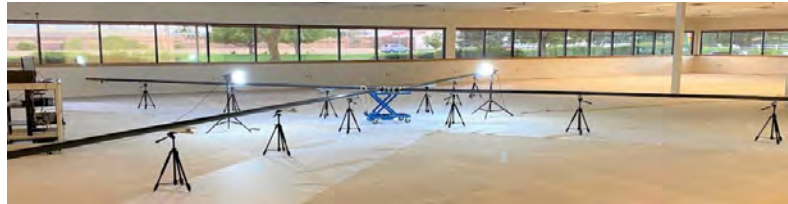
FIGURE 2. Four one-quarter scale composite booms were built and deployed from a prototype sail deployer.
