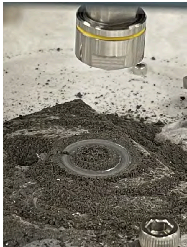
FIGURE 1. Three-body abrasion test on hBN-Al6061 coating using JSC-1A lunar simulant.
