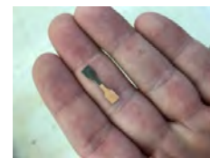
FIGURE 2. Subscale AM specimen built for tensile tests.
