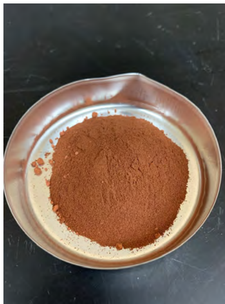
FIGURE 1. Mojave Mars Simulant 2 (MMS-2) Martian regolith simulant.
