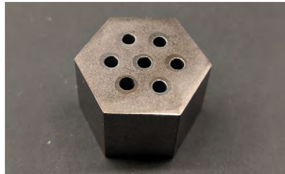
FIGURE 3. Sirius-2a cermet sample fabricated at MSFC.
