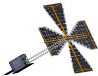
FIGURE 1. LISA-T PTD mission configuration. LISA-T array shown deployed from the 6U host CubeSat bus.
