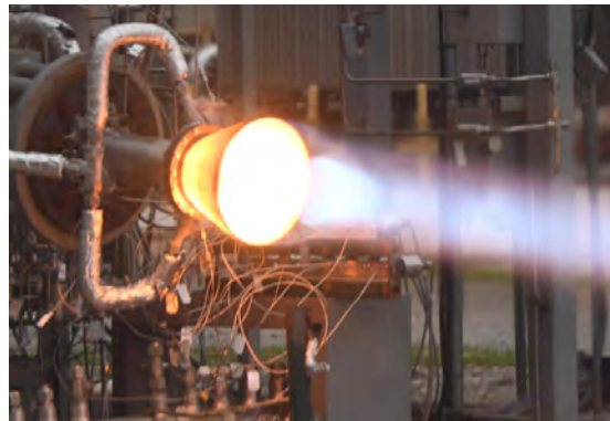
FIGURE 2. Hot-fire testing of a 7k-lbf GRCop-42 L-PBF thrust chamber tested at NASA MSFC Test Stand 115.
