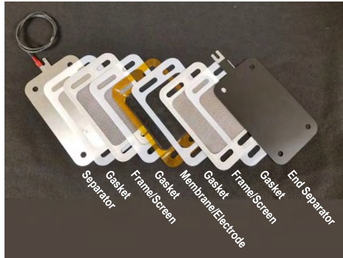
FIGURE 2. Expanded view of the electrochemical cell hardware.
