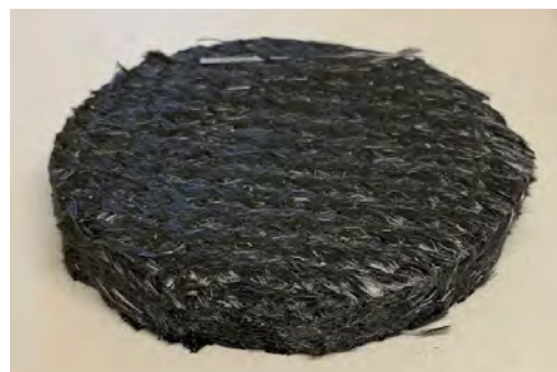
FIGURE 1. Shows a fresh, unused carbon fiber substrate.
