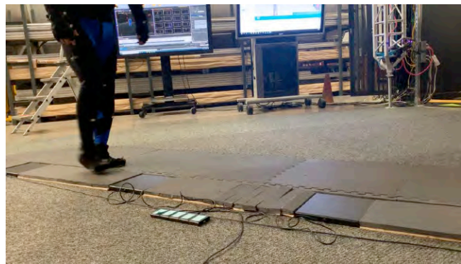
FIGURE 2. Phase I and II testing utilizing motion capture and force plate technologies.
