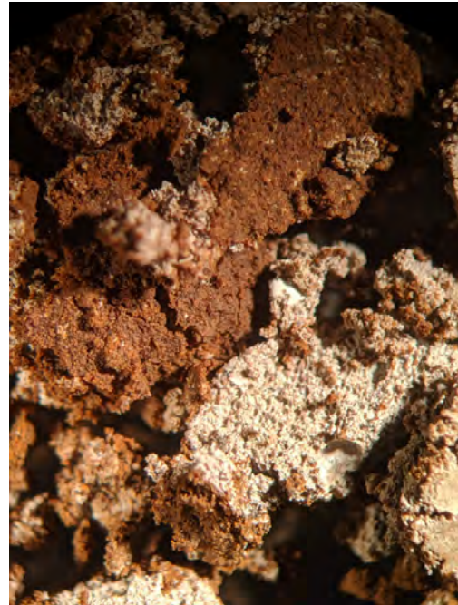
FIGURE 2. White precipitates indicative of silicates found on the surface of Martian regolith simulant after sintering with ILs.
