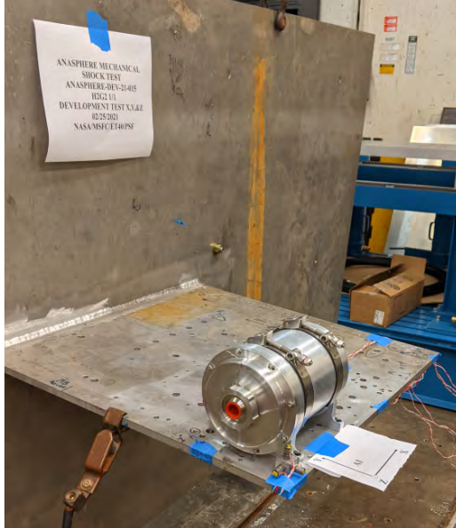
FIGURE 1. The small gas generator in the test rig for the shock test.
