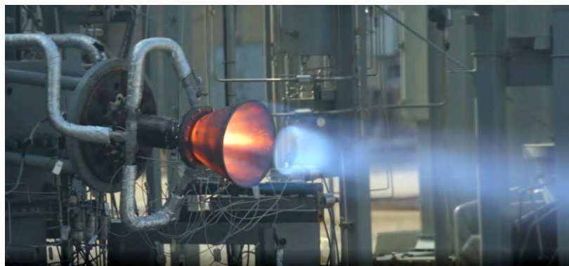
FIGURE 1. 7k-lbf AM GRCo-42 chamber with composite overwrap structural jacket completed testing at MSFC Test Stand 115.
