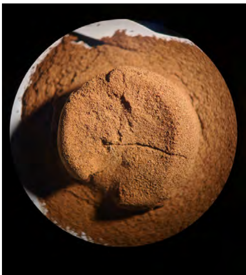
FIGURE 1. Martian regolith simulant after sintering with ILs.
