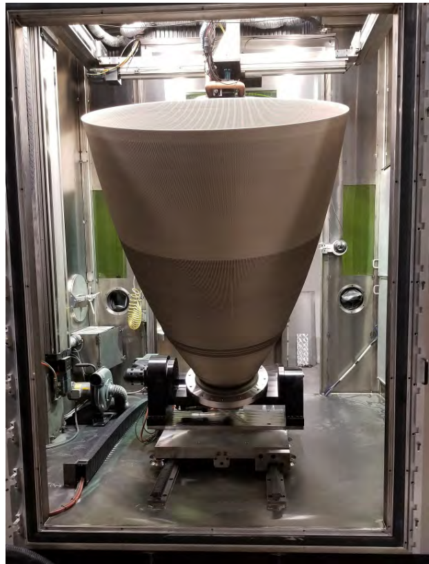
FIGURE 2. Ultra-large DED nozzle (58 in × 72 in) with integrated cooling channels that is ≈65% scale of the SLS Core Stage RS-25 engine nozzle. Build time: 90 days.
