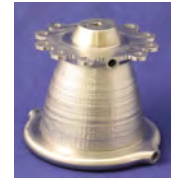
FIGURE 1. All-AM subscale nozzle with manifolds prepared for hot-fire testing.
