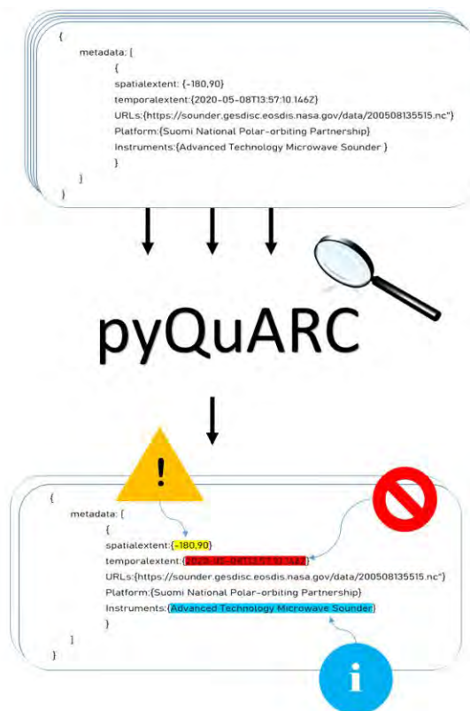
FIGURE 1. Conceptual diagram of pyQuARC. The Python-based library is designed to read and evaluate descriptive metadata used to catalog Earth observation data products and files.
