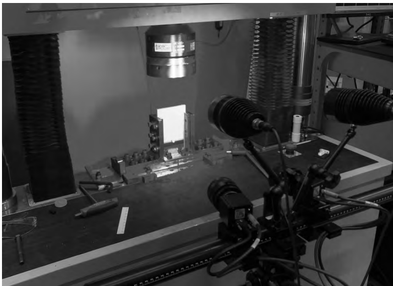
FIGURE 1. Pin-bearing test setup.
