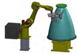
FIGURE 3. Demonstrated versatile methodology for automated closeout of large rocket engine nozzles.
