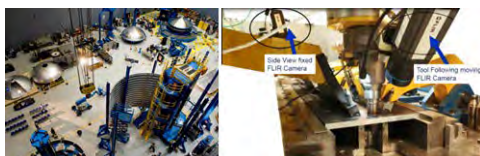
FIGURE 1. (a) MSFC South High Bay 4755 overhead view. In order to pre-production test welds, the use of (b) process development small-scale welding tools is also available. This validates the weld schedule(s) prior to actual (a) full-scale welding.
