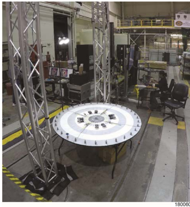
Figure 8. Over-all view of the radial-biaxial tensile test round table constructed at the NASA AFRC-FLL for radial-biaxial tensile tests of hyperelastic materials [under NASA New Technology Reporting protection (NTR) DRC-017-007].
