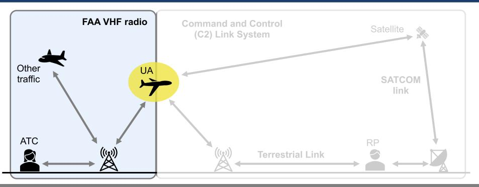
The current assumption is that unmanned aircraft (UA) talks with the air traffic controller (ATC) through the FAA's VHF radio, using the UA as a relay.
