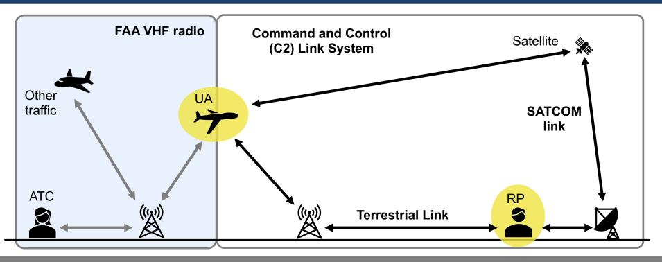
Then, the UA and the remote pilot are connected via the Command and Control (C2) Link System.
