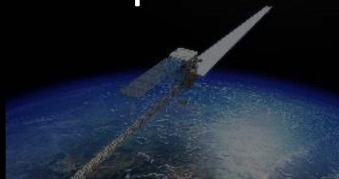
OSAM-2 will manufacture a beam and assemble solar arrays. Launch ~ 2023.
