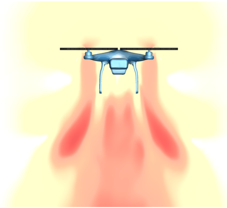
Figure 9. Velocity magnitude contours on a cutting plane through the centerline of a DJI Phantom 3 quadcopter in hover
