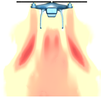
Figure 8. Stagnation pressure contours on a cutting plane through the centerline of a DJI Phantom 3 quadcopter in hover
