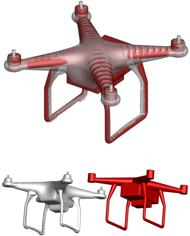
Figure 22. Comparison of laser-scanned DJI Phantom 3 geometry (light gray) with approximate fuselage composed of intersected geometric primitives (red). The geometries are presented overlaid (top) and offset (bottom) for clarity.
