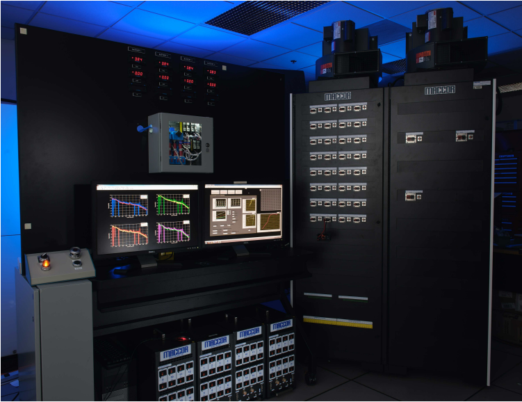
Fig. 2 MACCOR Battery Tester - Experimental Setup
