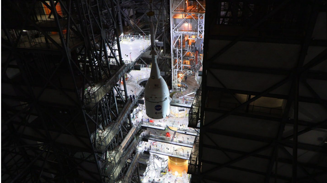
Figure 6: The Orion capsule is added to the Artemis I stack in the VAB at KSC on October 20, 2021.
