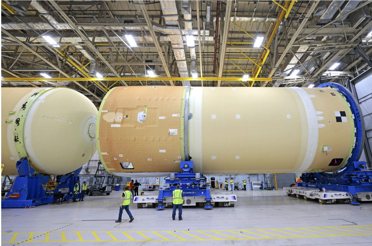
Figure 10: The Artemis II core stage forward join – consisting of the LOX tank, intertank, and forward skirt – is mated to the LH2 tank at Michoud Assembly Facility.
