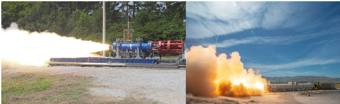
Figure 14: A subscale solid rocket motor test, left, at MSFC supports the evolved boosters, while a full-scale SRB test Utah, right, evaluates potential new materials and processes for missions beyond Artemis III.
