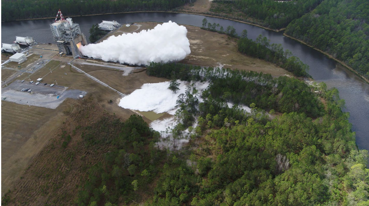
Figure 13: An RS-25 rocket engine is tested at SSC in February as part of the Retrofit 3a test series.
