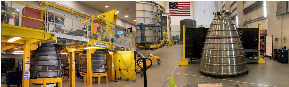
Figure 11: Two RS-25 engines for the Artemis III mission undergo inspection at SSC, left, and an RS-25 nozzle from the new production line for Artemis V and beyond, right.
