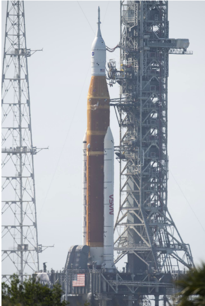
Figure 8: Liquid cryogenics vent from the Artemis I SLS during WDR.
