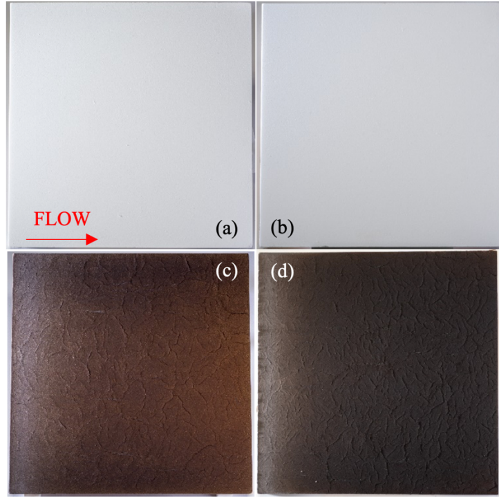
Fig. 23 (a) Pre-test PCC Acusil-II photograph and (c) post-test surface after exposure to Low condition (b) Pre-test PLGA Acusil-II photograph and (d) post-test surface after exposure to the High condition
