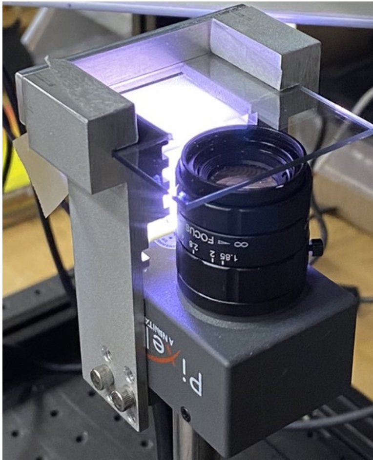
Figure 2: A photo showing the custom designed optics mount that attaches to the camera and contains the light source, opal glass, and Ronchi ruling. The mount is designed so that Ronchi ruling may easily be rotated 90 degrees by hand.
