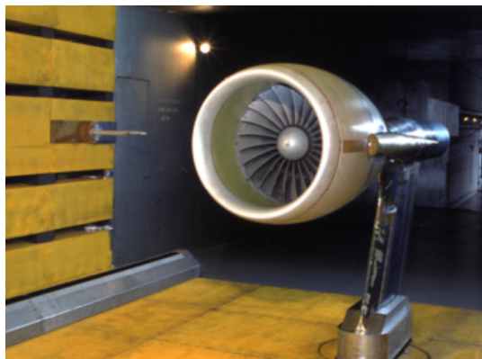
Figure 3 Inlet view of GE High Speed Fan model in GRC 9x15 LSWT
