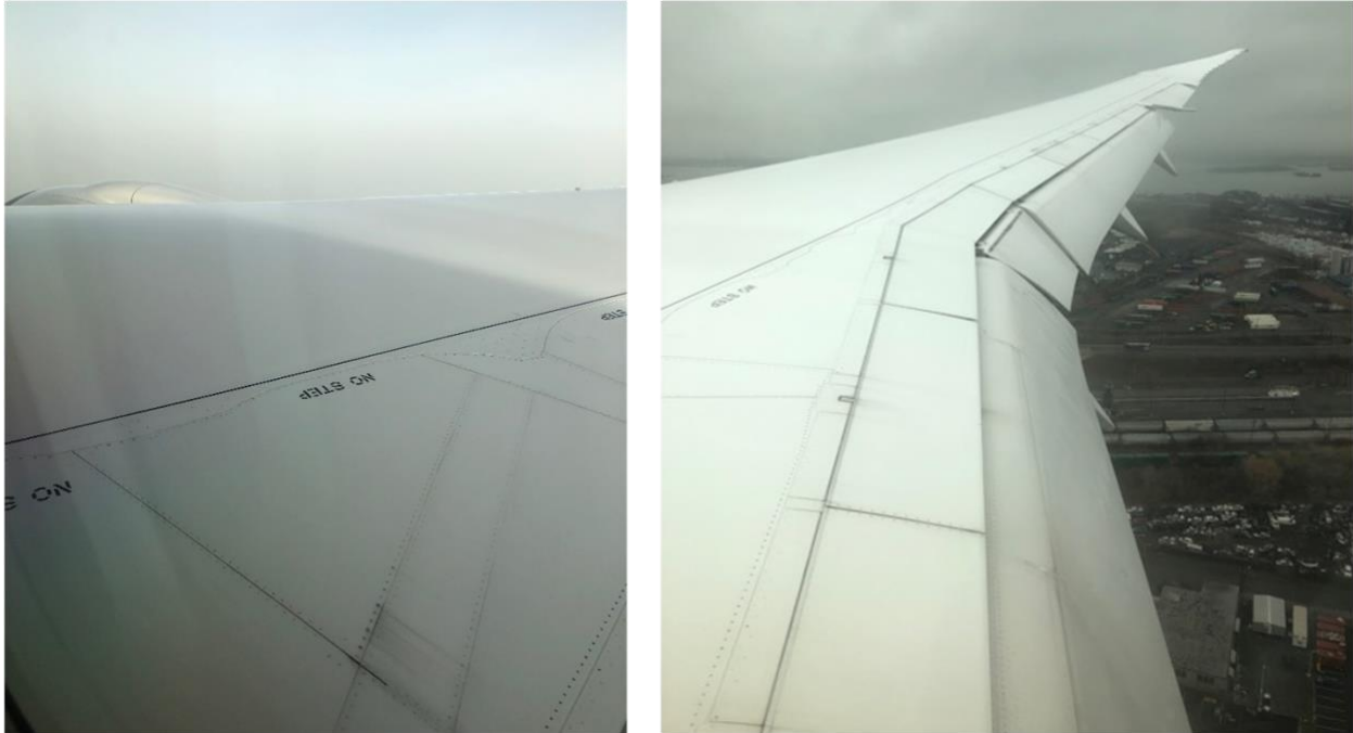
Fig. 3 View from above the wing of a Boeing 787-10 showing the wing as shielding engine noise by the leading edge (left) and aft-radiated engine noise by the trailing edge with flaps deflected (right). Photo Credit: Russell H. Thomas.
