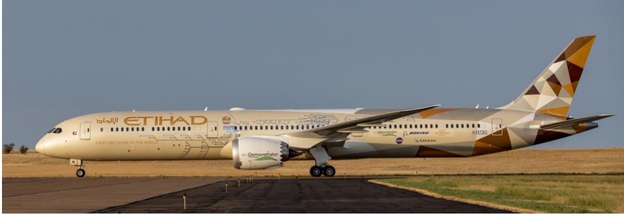
Fig. 6 Test aircraft outfitted with fuselage mounted microphones in four arrays: Over-wing, Under-wing, Axial, and Circumferential. Photo Credit: The Boeing Company.
