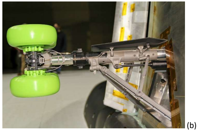
Figure 27. High-fidelity Main Landing Gear: (a) Position on Model, (b) Closeup View
