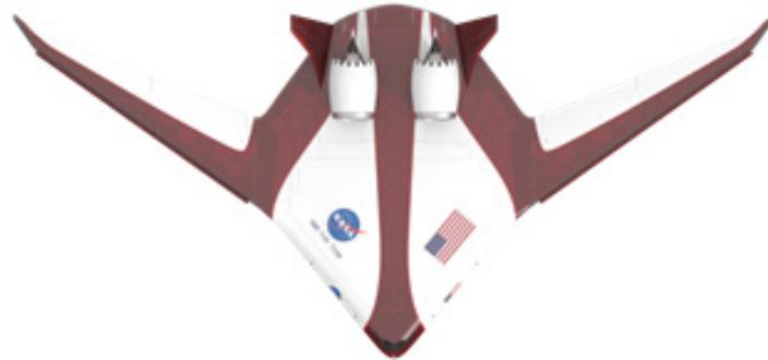
Figure 4.—NASA hybrid wing body concept airplane.
