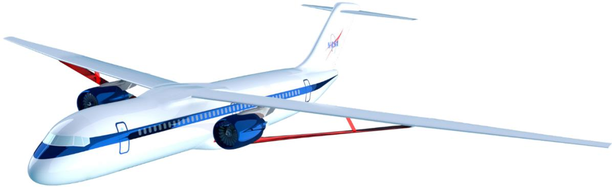
Figure 9.—Transonic truss-braced wing aircraft concept.
