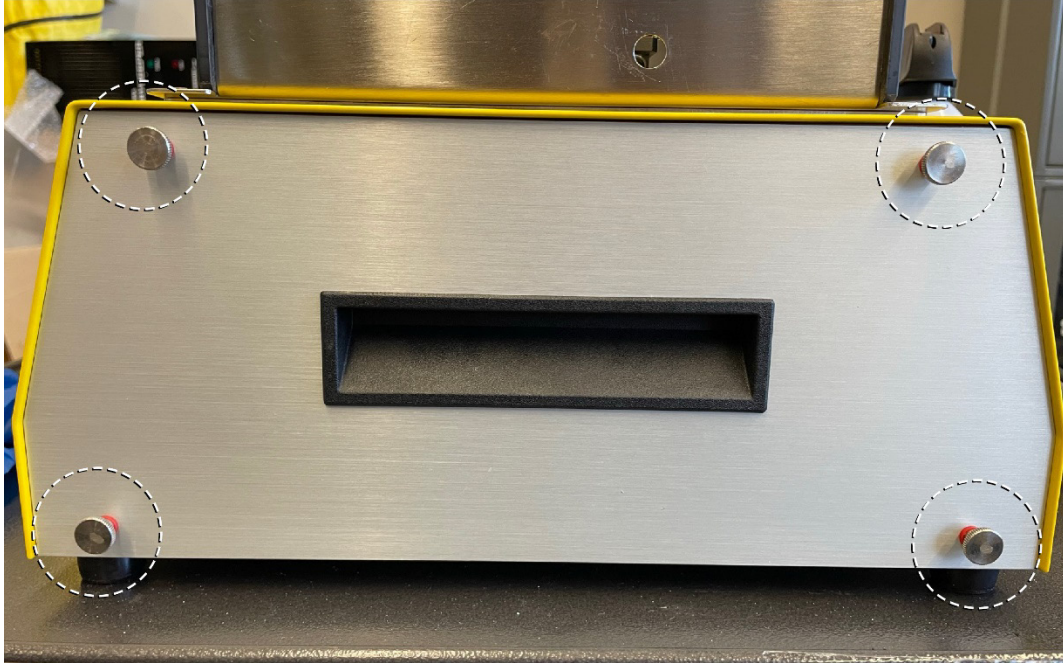
Figure C.2.—Detail of Step 4 showing thumb screws.
