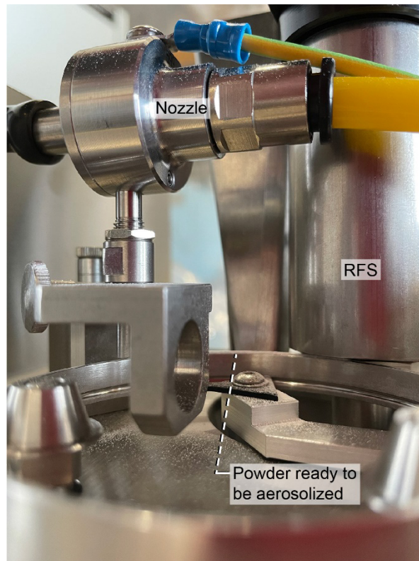
Figure 2.—Boehmite on dosing ring traveling to aerosolization nozzle. Reservoir and feed screw, RFS.
