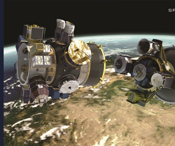
SPA-Ring Payload Port Limit (450 kg)
