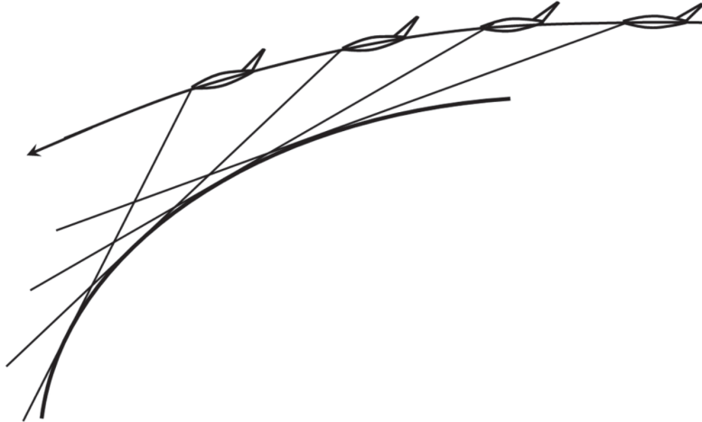
Figure 3-36: Caustic Due to Pushover (Source: NASA-CR-218871 [63]).
