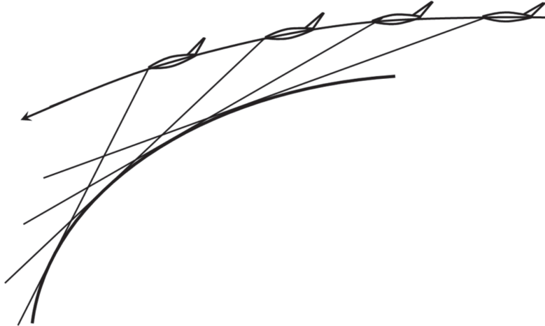
Figure 3-36: Caustic Due to Pushover (Source: NASA-CR-218871 [63]).
