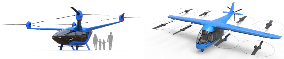
Figure 1: NASA RVLT reference vehicle configurations considered in this study: quadrotor (left) and lift plus cruise (right).
