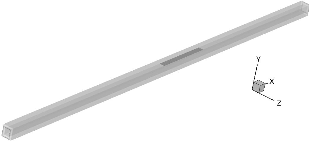
Figure 2. Modeling of an internal ducted environment as an external scattering problem. Liner section inside the duct is noted by the darkened area.
