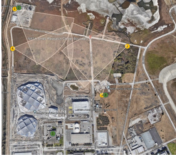
Fig. 2 Sensor's (yellow circles) and computing centers (green circles) locations on site the map.
