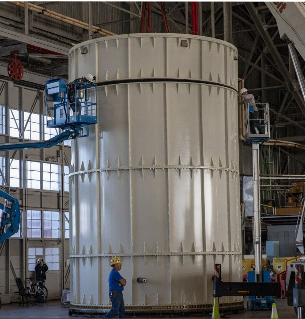
Orion mass simulator for integrated modal testing
