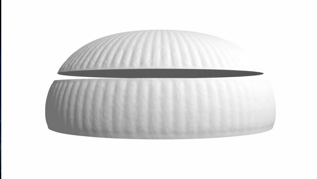
Flow over parachute in supersonic regime (particles colored by vorticity)
