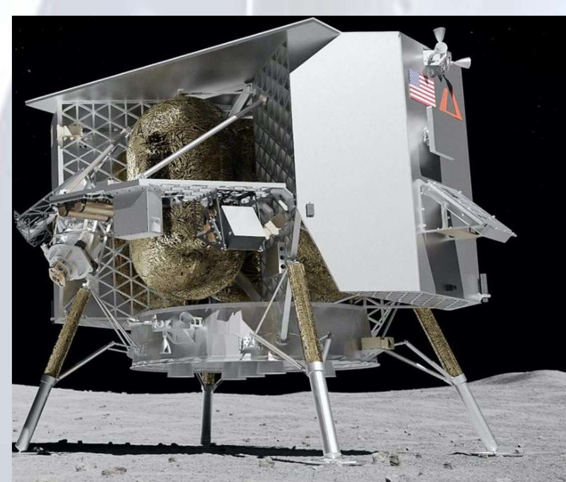
Left Image: Digital rendering of the Astrobotic Peregrine Lander. PILS is mounted on the right side of the spacecraft. Image Credit: Astrobotic, image used with permission.
