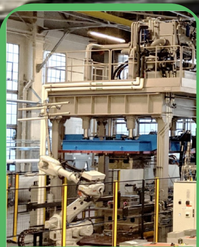
PREFORMER LINE (aka Small Press) Max Force 330T
