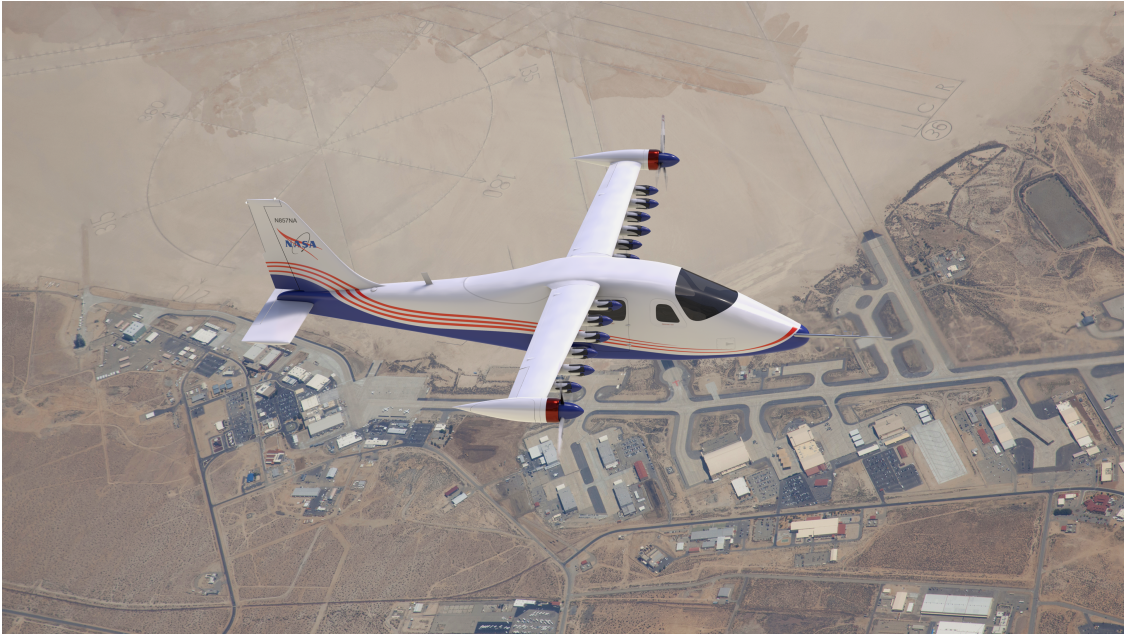
Figure 4.9: An artist's rendering of the X-57 Maxwell aircraft in flight, shown in the Mod IV Configuration.
