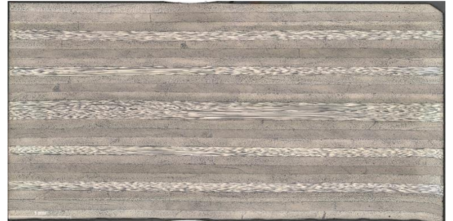
LM-PAEK ICAT + Autoclave post-consolidation
