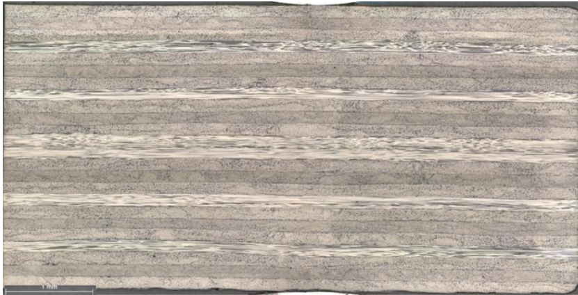
PEEK ICAT + Autoclave post-consolidation
