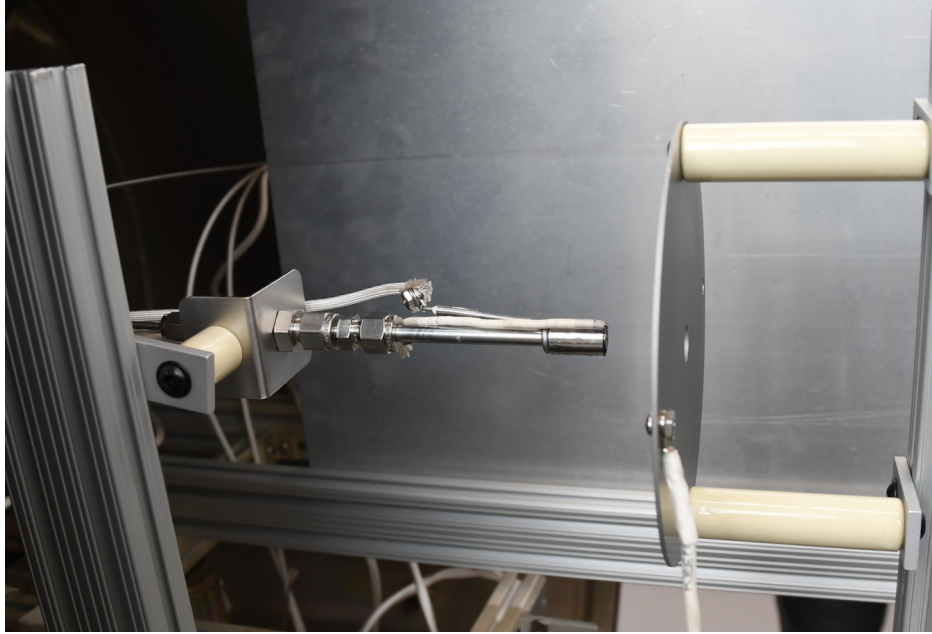
Fig. 1 A test cathode installed in VF-67. The plate anode is on the right. The second cathode is located behind the metal divider.
