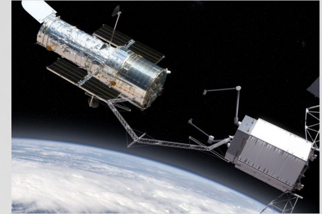
Tendon-Actuated Lightweight In-Space MANipulator (TALISMAN)
