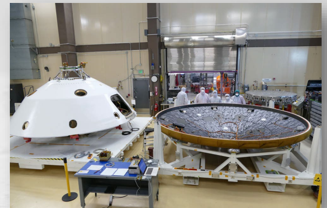
Mars Entry, Descent and Landing Instrument 2 (MEDLI2)
