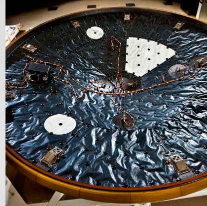
Mars Entry, Descent and Landing Instrument 2 (MEDLI2)
