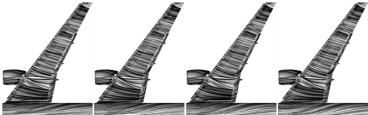
(a) Baseline (Free-Air) (b) With Standoff (c) With Standoff + Thin BL (d) With Standoff + Thick BL
