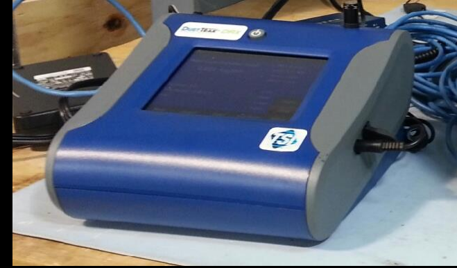
Example of a mass concentration aerosol instrument, DustTrak DRX (cal factor required)
