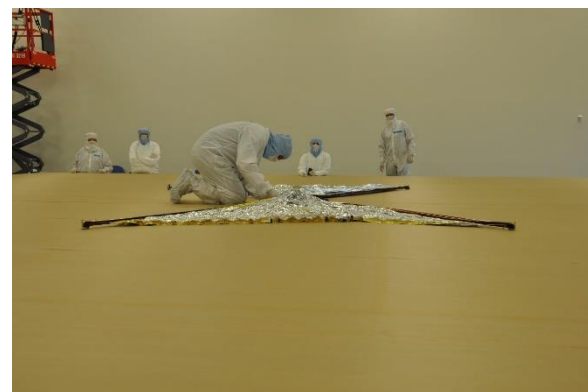
Figure 7: NEA Scout’s flight sail unfurls in a bowtie configuration during a deployment test
