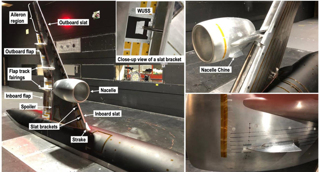
Figure 3. Photographs of CRM-HL model with the engine nacelle (baseline, left) and with nacelle chine installed (upper right). A close-up view of the nacelle chine is on lower right.
