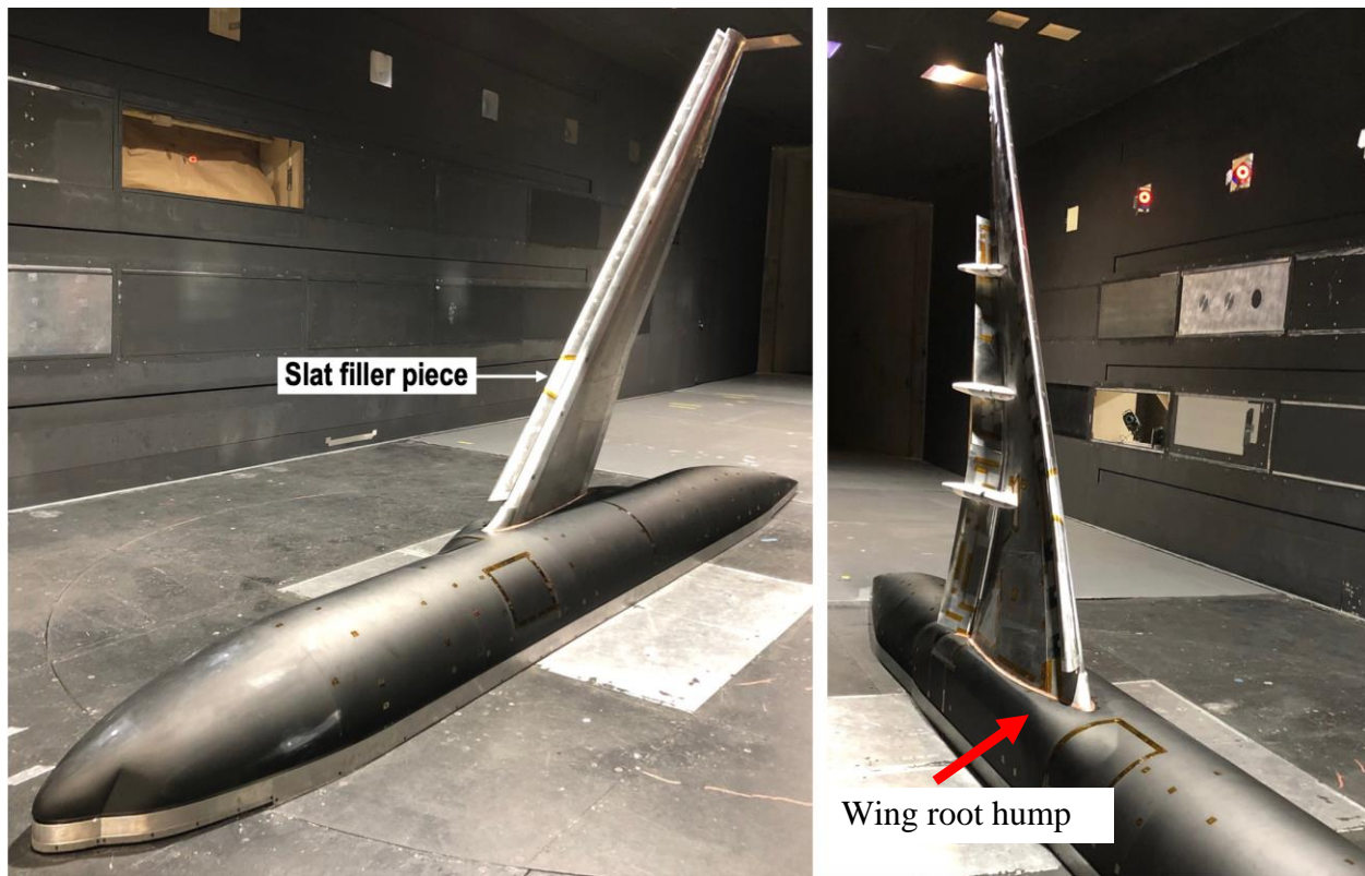
Figure 5. Photographs of CRM-HL model without engine nacelle: upper surface frontal view (left) and lower surface frontal view (right).
