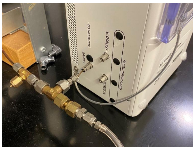
Figure 9. Science Verification Testing (SVT) setup, in which the test mixtures are sampled by the AQM in a slip-stream approach. In this configuration, the purge inlet pulls from the laboratory air, which is at a lower concentration than the elevated transient concentrations experienced by the sample inlet.
