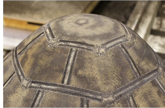
Fig. 7: HEEET dual layer integrally woven TPS Engineering Test Unit (tiles configuration with 2 rings of flank tiles)
