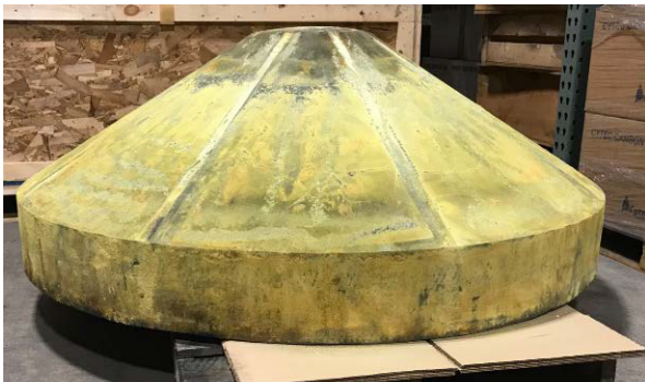
Fig. 4: Domestic lyocell 1.4m single piece PICA demonstrated to support future NASA opportunities including sample return missions
