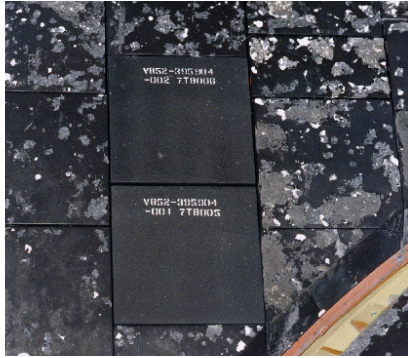
Fig. 1. 2 TUFROC coated tiles provided improved impact damage / toughness compared to RCG coated tiles.
