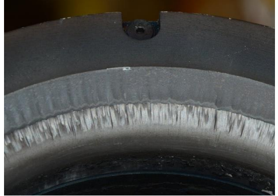
Fig. 8. Striations observed on the outer chamfer of the NASA-103M.XL after 4,731-hour of operations.
